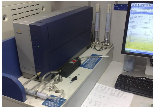
Figure 2.13: A typical ultra-fast Gas Chromatograph utilised in a Queensland underground coal mine [15]
