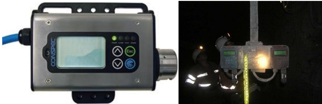
Figure 2.10: Installed real-time gas detector in a Queensland underground coal mine [48, 51]
