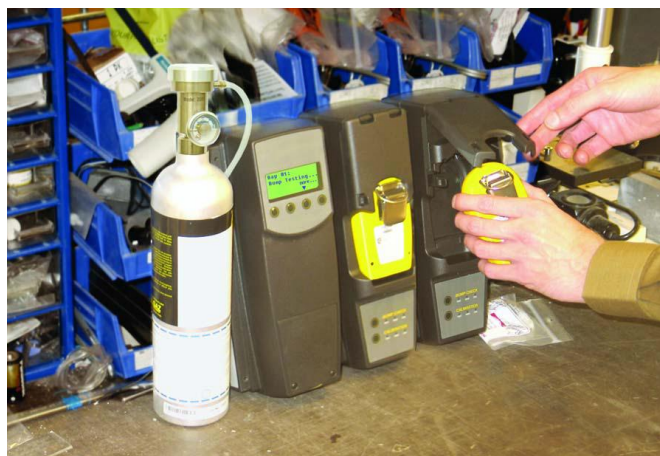
Figure 2.8: Calibration of catalytic instrument for different gases [12]
