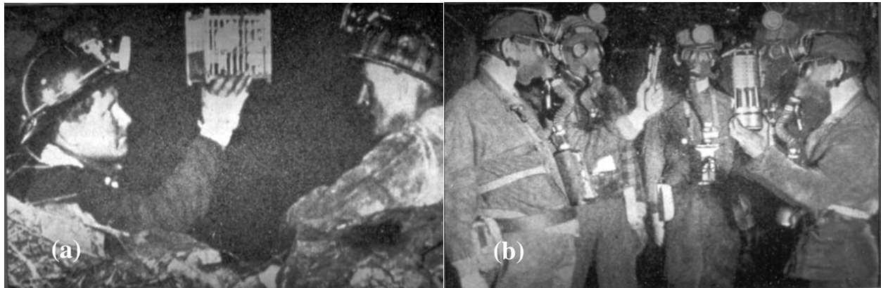
Figure 2.1: (a) Canary bird in cage, and (b) safety lamp for gas detection in underground coal mine [11]
