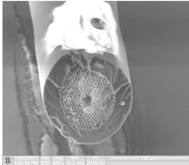
Figure 7.12: Scanning electron micrograph (SEM) showing the cross section of a hollow core fibre that has had a 10 \mu\text{m} dia. hole drilled into its core (the fibre tip was broken)
